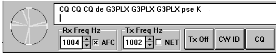
Fig. 6 Screenshot of the control panel of the PSK31 WINDOWS program, with the tuning display showing a slightly noisy QPSK signal, and showing the fine-tuning controls for the receive and transmit audio tones.
