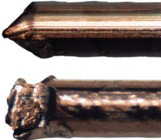
(Effects on center conductor when cut by a pair of diagonals)
